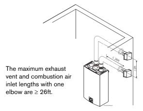
Fig. 9 Maximum vent and combustion air lenghts
